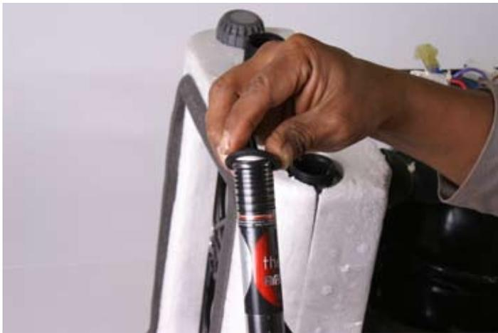
Place o-ring over the top of the Heater and push down approximately 3/4 inch to 1 inch onto the Heater.
