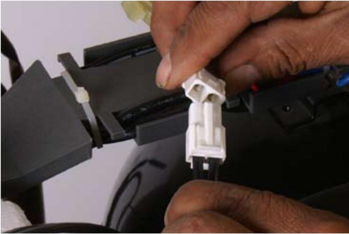
Connect two pin adapter on wiring harness to two pin connector mounted on top of support strut.
