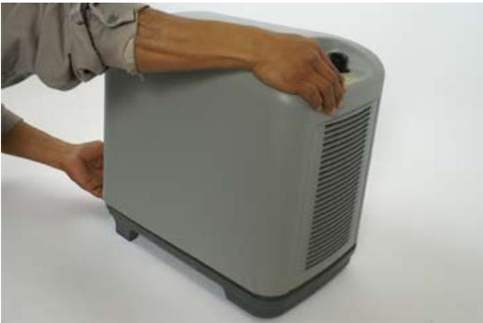
Pull upwards on rear of chiller housing, loosening it on the frame of the chiller.
