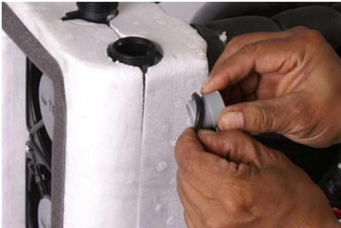
Remove plug and o-ring from ring nut.
