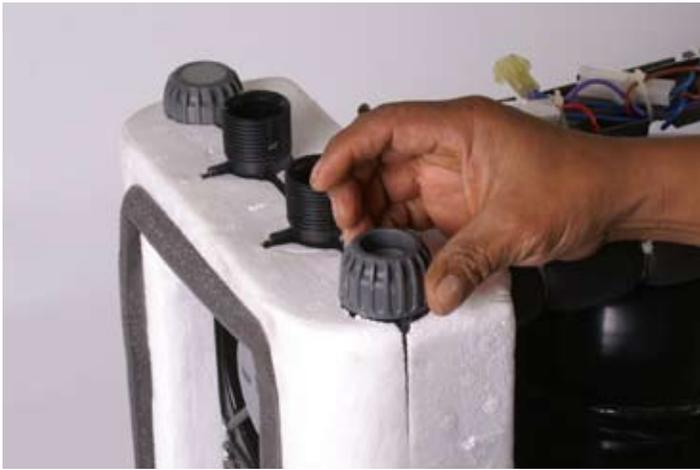
Unscrew and remove ring nut over Heater port.
