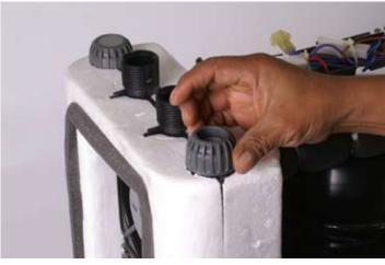
Remove plug and o-ring from ring nut.
