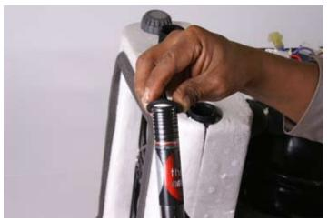
Insert Heater into heat exchanger until o-ring seats into outlet lip. If you encounter resistance while inserting the Heater, gently turn the Heater and apply very slight force.
