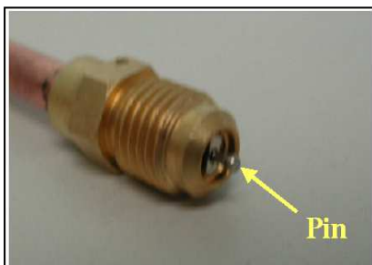
Pict.1: This picture shows the pin inside the valve hole.
