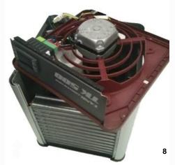
Remove the red or grey fan support lifting it up from the bottom edge.
