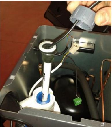
Disconnect the heater connector (img.22)
