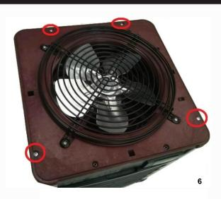
Using the screw-driver, remove the 4 INOX screws indicated in the picture
