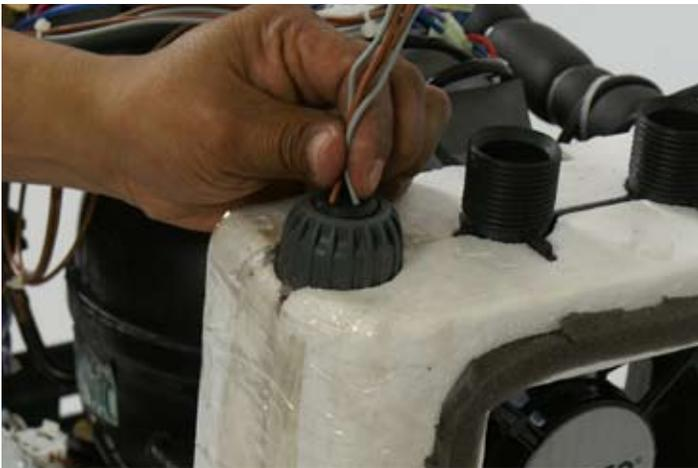
Push plug firmly into quartz sleeve until it is flush with the top of ring nut.
