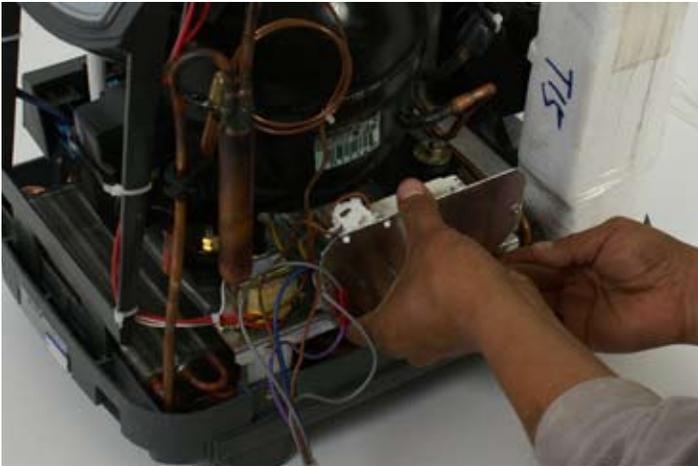
Line the holes in the ballast mounting plate with the holes in the strut supporting the compressor.
