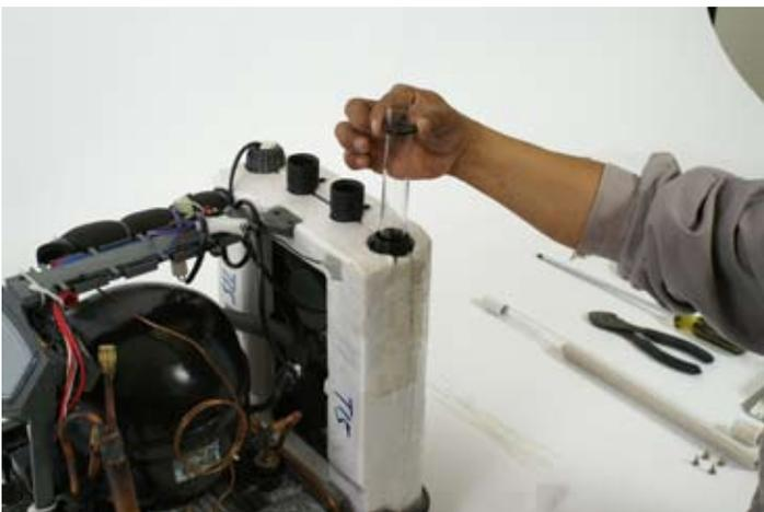
Insert quartz sleeve into heat exchanger until o-ring seats into outlet lip. If you encounter resistance while inserting the quartz sleeve, gently turn sleeve and apply very slight force.
