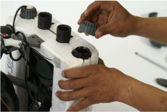
Unscrew and remove ring nut over UV port.
