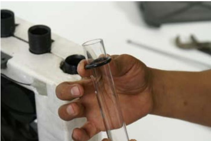
Place o-ring over the top of the quartz sleeve and push down approximately 3/4 inch to 1 inch onto the quartz sleeve.
