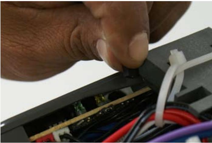
Place Jumper over pins 2&3 (see diagram below)
