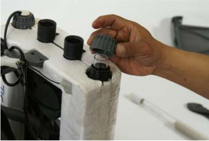
Put ring nut over quartz sleeve and o-ring. Tighten to seal.
