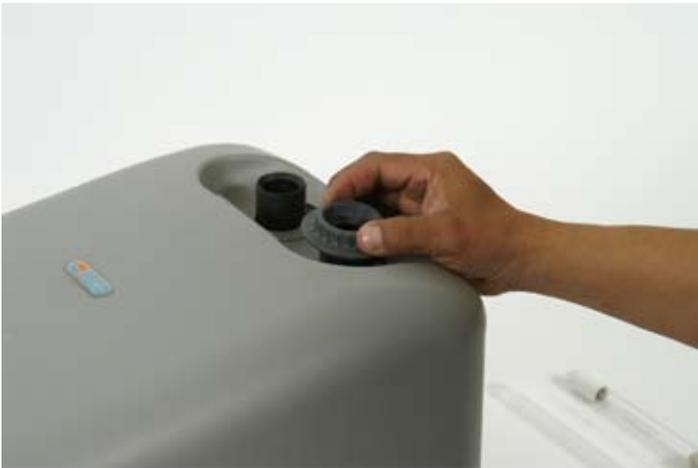
Once loosened, manually remove the plastic nuts.
