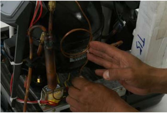
Carefully bend the copper capillary tubing to make space for the ballast. It is helpful to look ahead and see where the ballast will mount to determine how to move the tubing. Be careful not to crimp or break the tubing.
