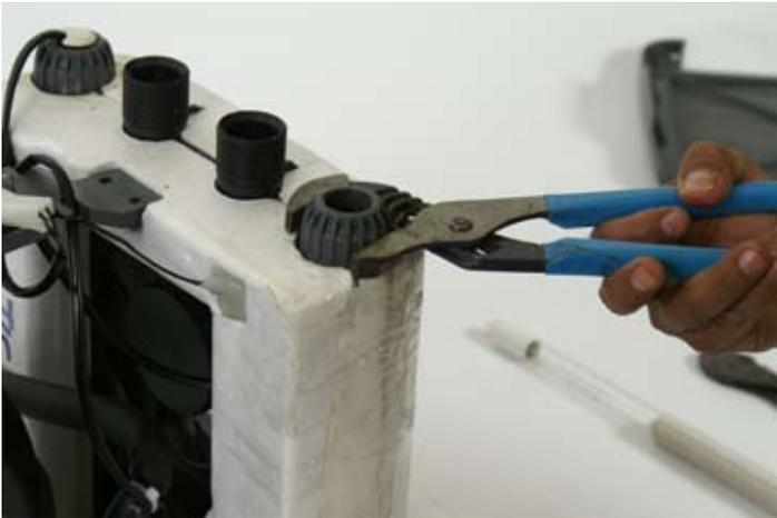
Use channel lock pliers or similar to insure there is no leak.
