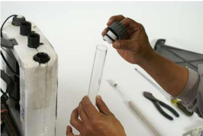
Remove plug and o-ring from ring nut.
